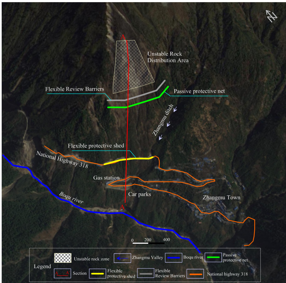
Fig. 13 Schematic layout of rockfall prevention measures.
