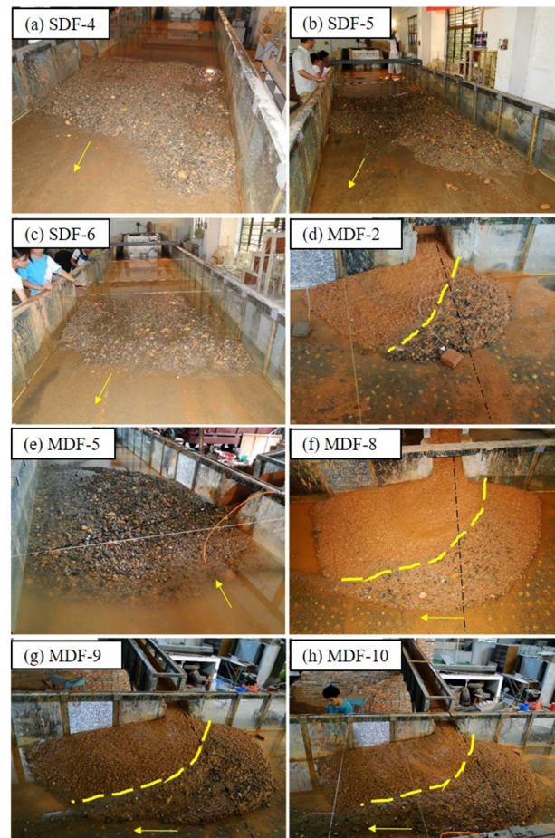
Fig. 6 The surface features of the depositional fan of SDF (stony debris flow) and MDF (muddy debris flow): (a, b and c) downstream view of depositional fans in tests SDF -4, -5, and -6; (d) frontal view of depositional fan in test MDF-4; (e) upstream view of depositional fan in test MDF-5; (f, g and h) frontal view of depositional fans in tests MDF-8, -9 and -10. The yellow arrow indicates the water current direction, dot-yellow line marks the boundary of fan with and without water scouring.
