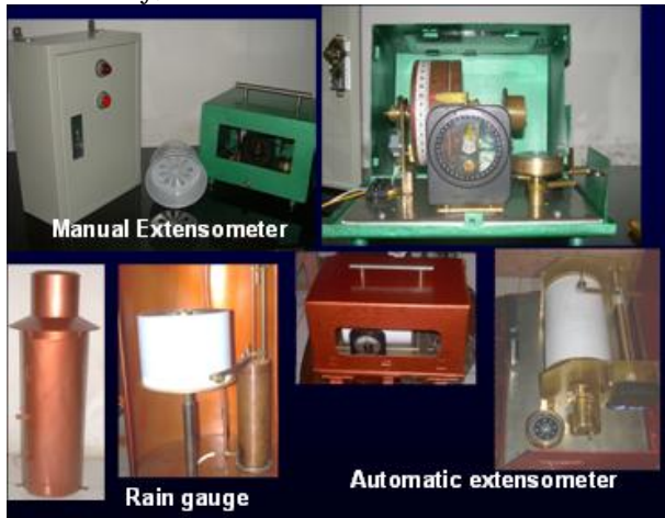
Figure 7 Early warning system equipments consisting of a) manual extensometer with the control panel and sirene and b) rain gauge, developed by Fathani et al. in 2008.
